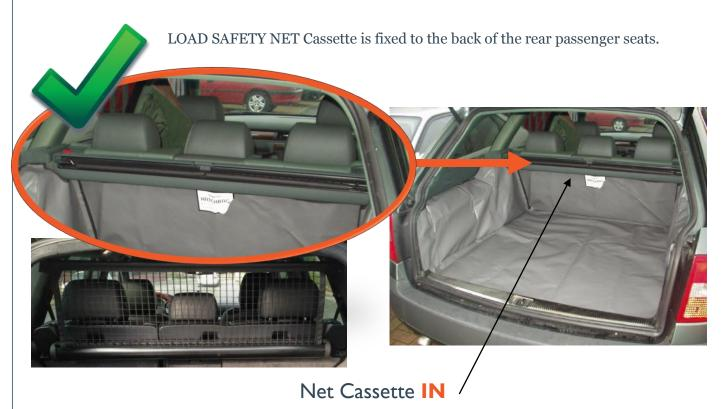
The Bootliner panel that sits against the back of the seats finishes just under the cassette and fixes to the under face of it – you can NOT remove the cassette whilst the liner is in place.
