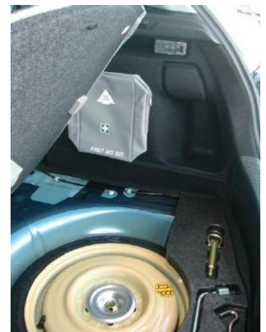
The space saver wheel sits directly under the carpet base.
