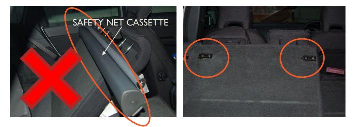
The Safety Net Cassette fixes to the back of the rear seats, prohibiting the use of the boot liner headrest straps.
