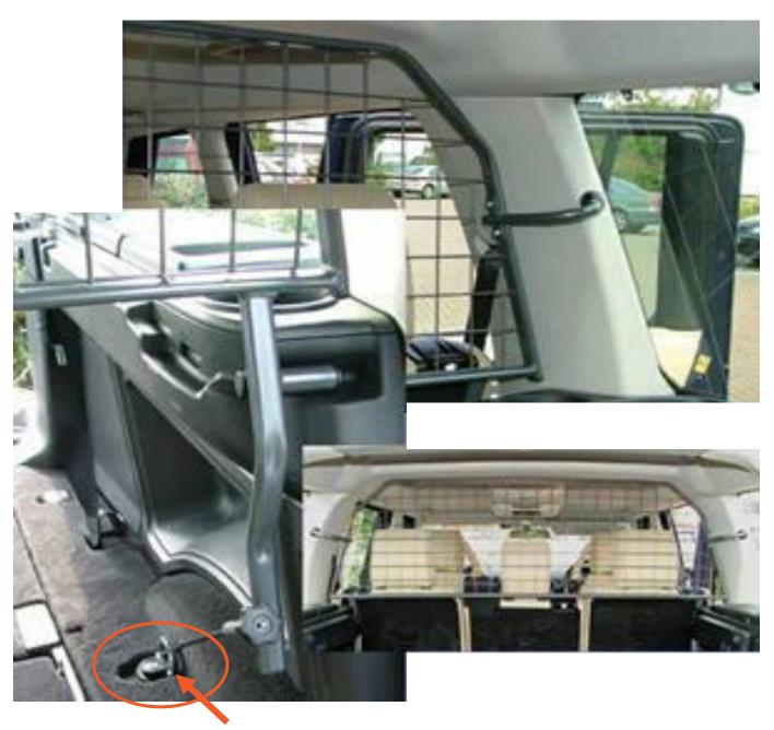
$Cut \ outs \ provided \ in \ the \ boot \ liner for \ these \ floor \ fixing \ points \ that \ highlighted$
