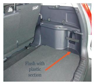
The liner has been designed with the  $2^{nd}$  tier false floor (See photo A) stored at the lowest level. (See photo B) The  $2^{nd}$  row seats are to be slid as far back to the tailgate as possible.
