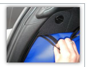
Fold the pocket flap over the net, and tuck behind the wheel arch.
