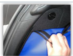
• The 2 rear "D" rings are accessible: Two bound slots in the side panels provide access to these fixing points.
