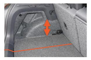
Floor is raised to sit almost flush with the tailgate plate.
