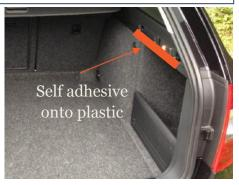
REAR END Self-adhesive loop fastener onto plastic
