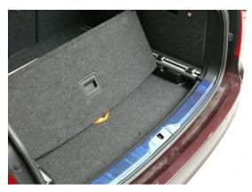
The false floor can NOT be folded open when the liner is in place
