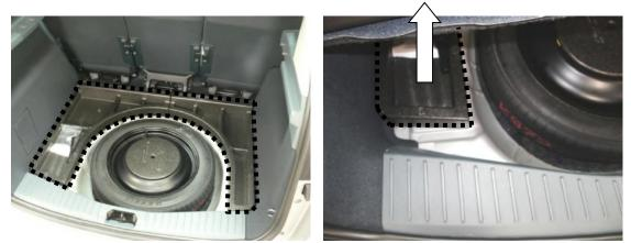
3. Re-place the Carpeted Floor panel with the back edge butted up to the metal tailgate plate.
