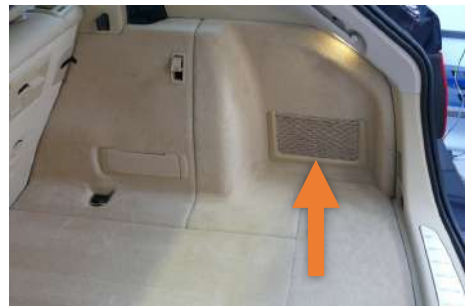
Right side net flush to side wall
