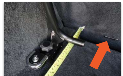
Ties fasten to these metal loops
