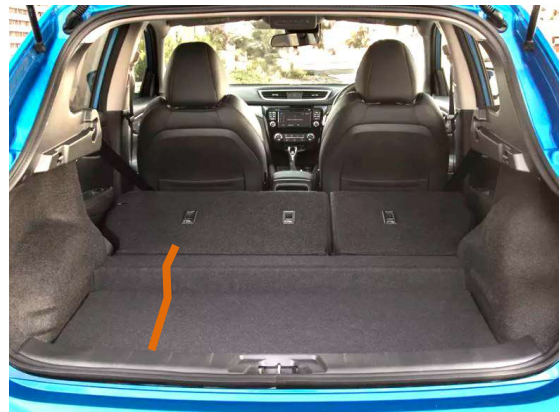
Floor steps down from behind the rear seats
