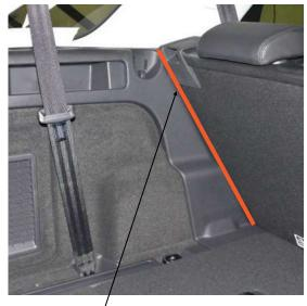
When the seats are most reclined there is no void between the seat upper and the plastic molding
