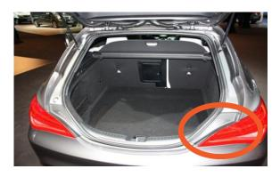
Smaller boot aperture: entire rear light cluster still visible when boot door open
