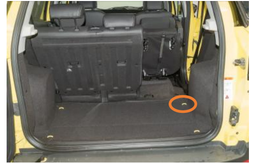
No false floor & D-Rings are exposed
