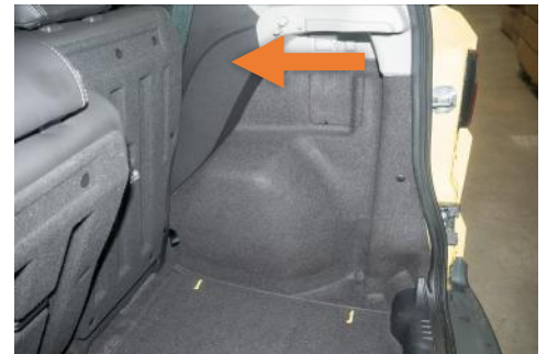
Offside - rear seats do not lock into D-Ring mounted onto plastic boot side
