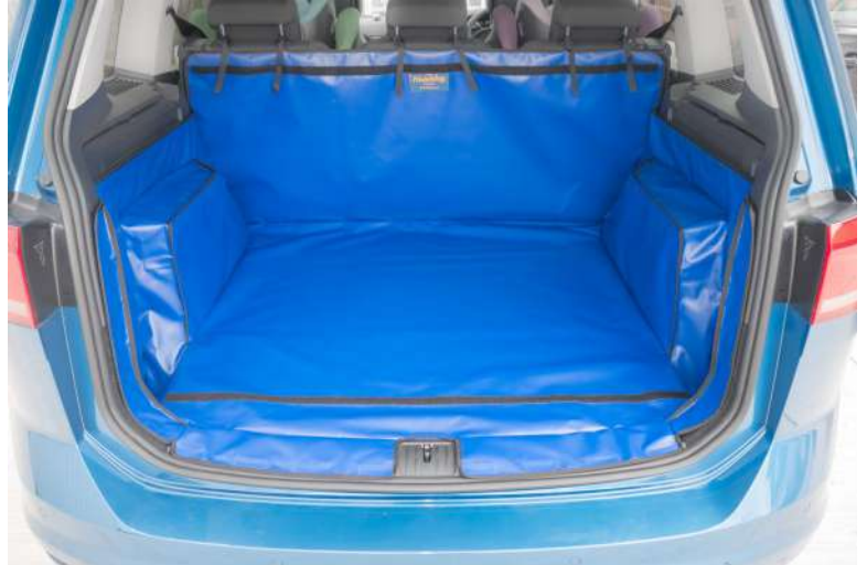
Standard boot liner with seat flap and bumper flap prep
