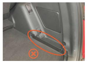
The boot liner does not accommodate these separators, they need to be removed from the vehicle before fitting.
