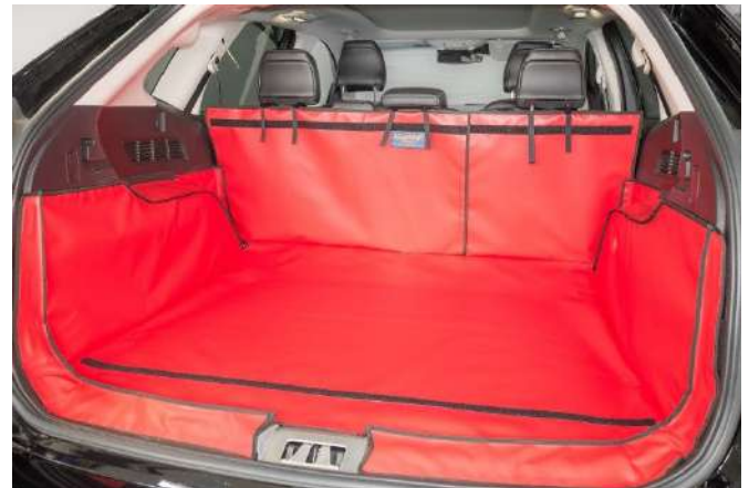
Photo shows a Rear Split boot liner prepared for an additional Seat flap and Bumper flap
