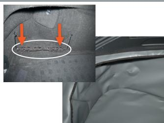
H0698-NET2 AVAILABLE NET ON BOTH SIDES The liner will be cut to accommodate both nets. (following the blue line).
