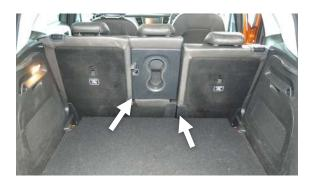
Seats must be slid as far back to the tailgate as possible and set to the fully reclined position.
