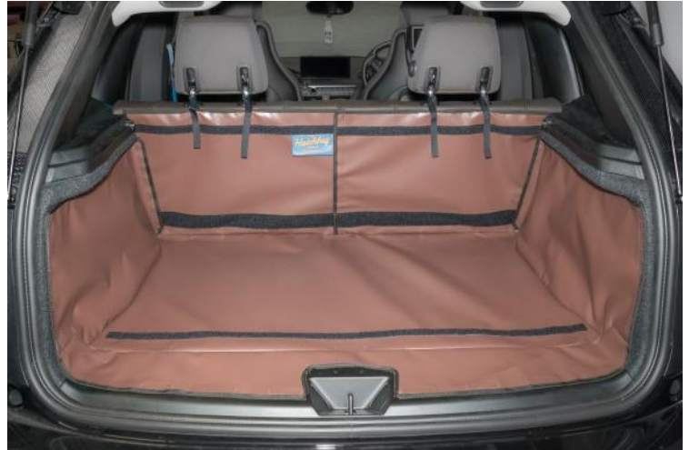
Split boot liner prepped for a seat flap and bumper flap and boot liner extension
