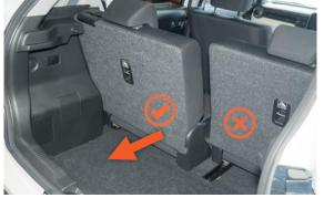
Rear seats must be fully reclined & fully pushed back towards the tailgate H0721-SE5
