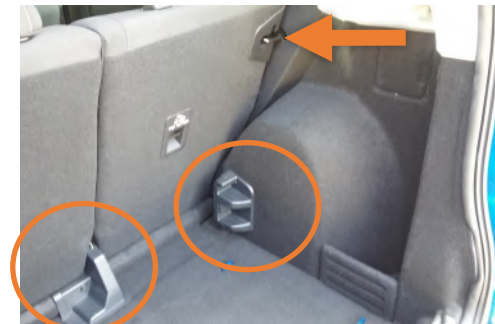
Plastic mountings & modified seat lock with D-Ring mechanism
