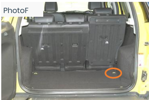
No false floor & D-Rings are exposed
