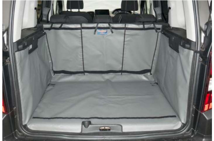
Rear split boot liner prepped for seat flap, floor extension and bumper flap
