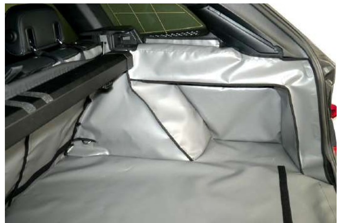
HYNO Rear Plus with Seat Split boot liner with additional D-ring access and prepped for a bootliner extension and bumper flap
