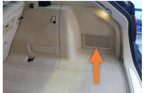
Right side net flush to side wall
