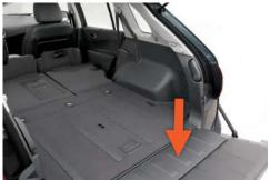
Split rear door - Lower section drops down & sits flush with boot floor
